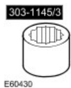
Camshaft pulley bolt socket 303-1145/3
