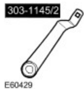
Camshaft pulley bolt remover 303-1145/2
